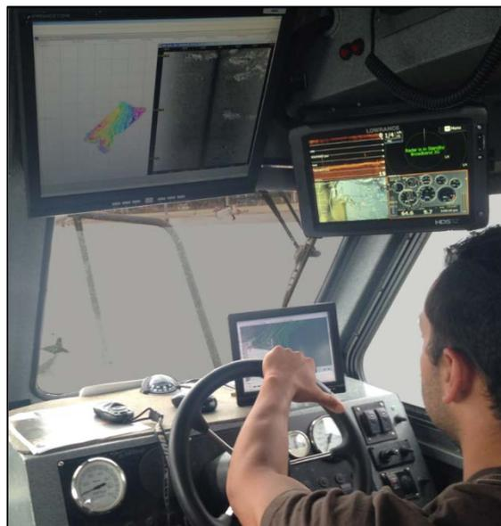
**Survey vessel used to map eelgrass and provide bathymetric and sidescan waterfall data.**
