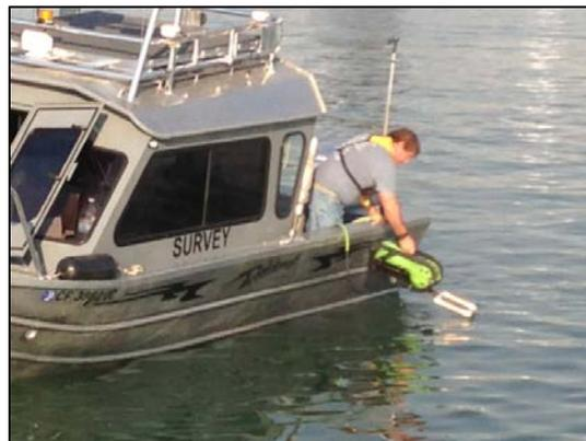
**An ROV was used to ground-truth acoustic records and collect eelgrass shoot density data.**
